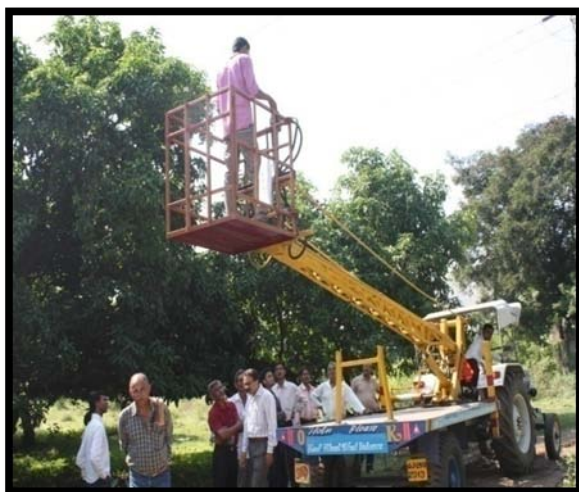
Demonstration of Tractor Trolley Mounted Hydraulic Platform and Power Sprayer
