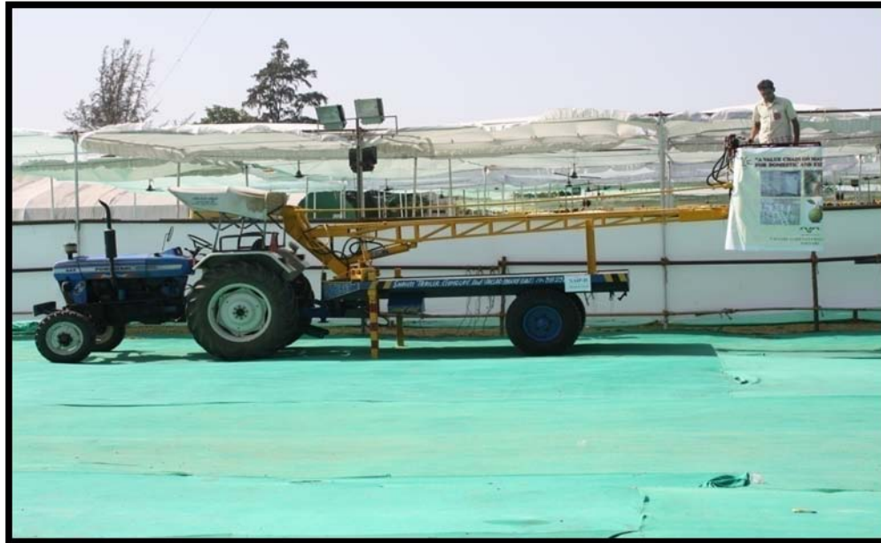
Demonstration of Tractor Trolley Mounted Hydraulic Platform at Krushimela -2010.
