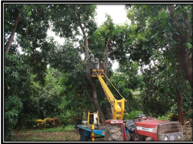
Use of Tractor Trolley Mounted Hydraulic Platform by Farmers for spraying and pruning in Mango Orchard
