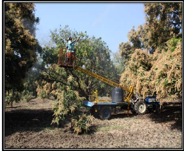
Use of Tractor Trolley Mounted Hydraulic Platform by Farmers for spraying and pruning in Mango Orchard
