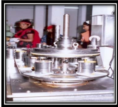
Mango Pulp Can Filling and Seaming Unit
