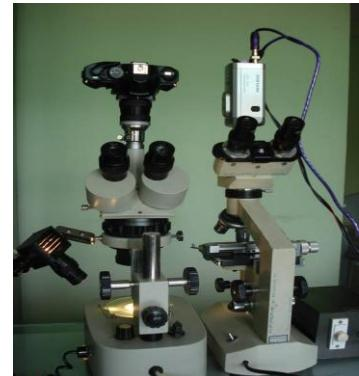
Stereotriangular and research trinocular microscopes with CCD camera and photomicrographic attachments
