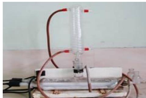
Doble distillation apparatus
